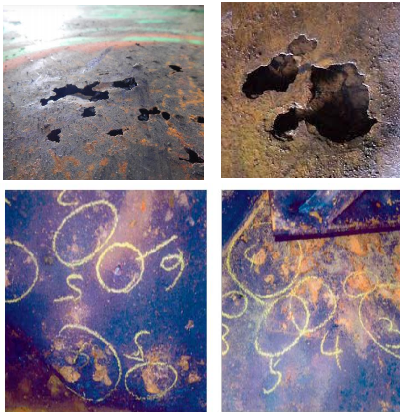
Examples of storage tanks damaged by localized corrosion
