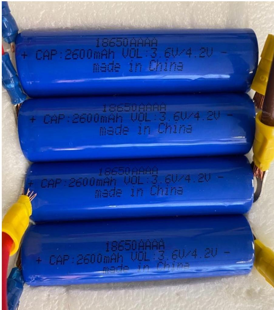
The cells used are 18650 lithium-ion type
